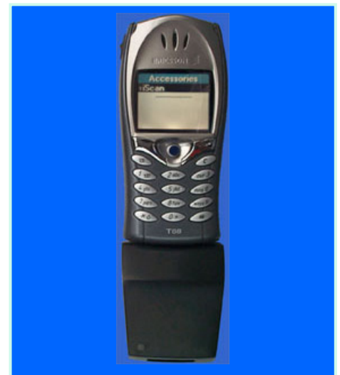
IScan's shopping technology is based on a conventional mobile handset fitted with a barcode reader.
