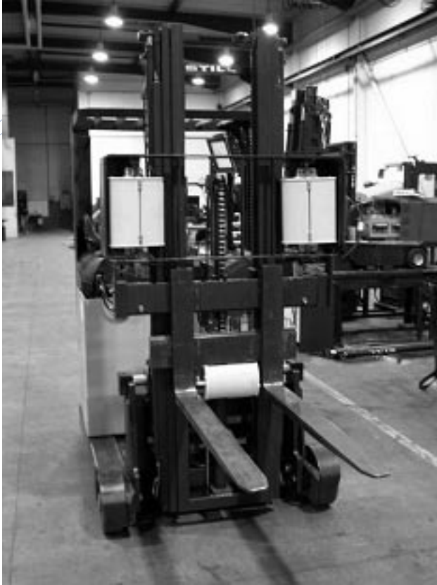
Figure 7: Forklift Mounted Interrogators
